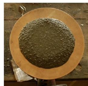
*1:6 Mfd. Sand mortar at 85%flow*
