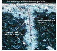
steel. Once the passive film is destroyed, the affected portion of reinforcing steel is exposed to action of oxygen and water; consequently, corrosion in reinforcement steel is initiated.
