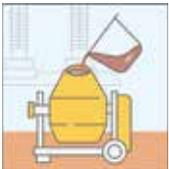
Add the WP+200 water mixture to the prepared concrete, plaster or mortar mix.
