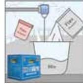
Mix the powder and liquid polymer ensuring lump free consistency, preferably using a mechanical stirrer.
