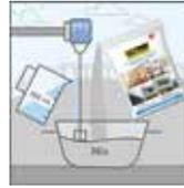
Add 1 kg powder to 350-380 ml of water and mix well to get a lump-free consistency, preferably with a mechanical stirrer.
