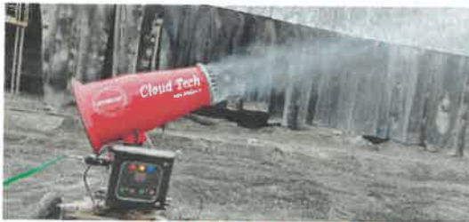
Fogging system at Railway Siding
