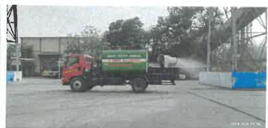
Truck mounted fogging system
