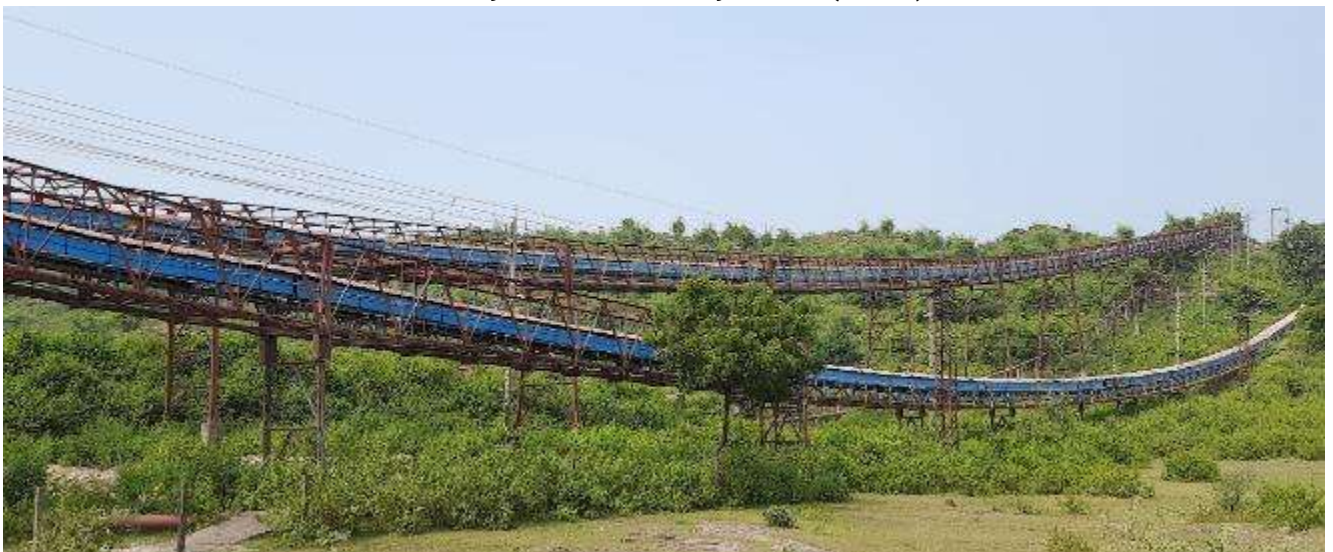
Fully covered Conveyor belt (OLBC)
