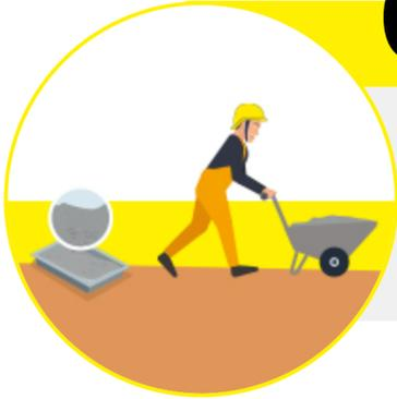
While transporting the mixture, there should be no jerks, the concrete should be placed in the shuttering within 30 minutes of pouring water in it.
