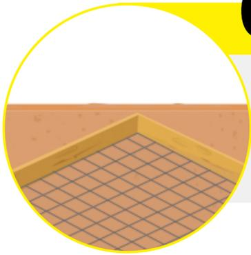
Take note that, while placing the concrete, the alignment of the formwork should not be disturbed or shaken.
