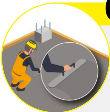
The last step is trowelling, in which the steel trowel is used. This helps you in giving very smooth, uniform surface.
