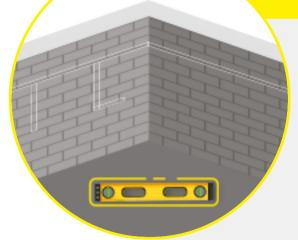
First of all, mark the points for taps, showers, wash basins and the way for the pipes connecting to them on walls. You can use spirit level for this.
