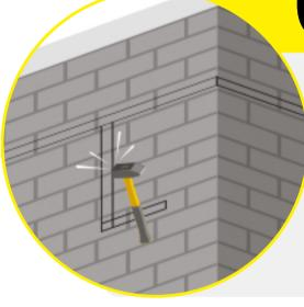
For making grooves, cut the portion between the two lines with the help of a shovel; if the wall is load bearing, do not cut it at one time.
