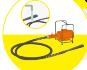
Be sure to clean the needle and shaft pipe after work.
