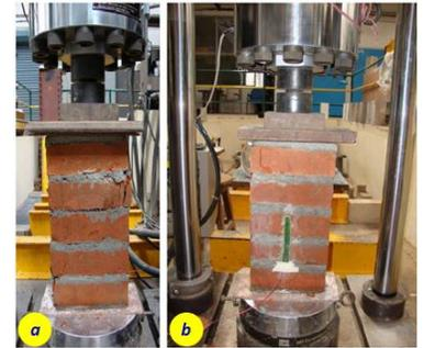
Stack bonded masonry prism under compression test
