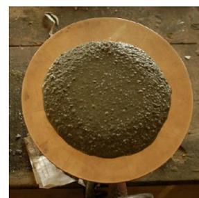
*1:6 Mfd. Sand mortar at 85%flow*
